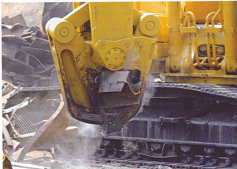
Patented Allied-Gator MT Series Multi-Tool model MTR 70 with patented Quick-Change Shear Jaw Set – processing a heavy I-beam.
