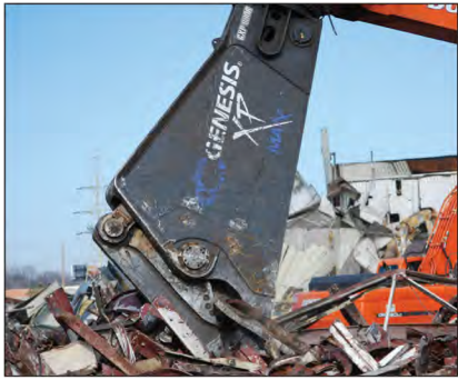
The Genesis XP shear employed in a scrap application. Photo courtesy of Genesis
