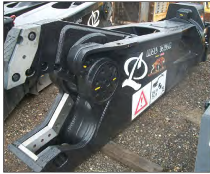
The Stanley/Labounty MSD1500 mobile shear. Photo courtesy of Company Wrench
